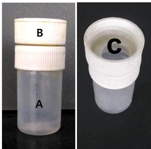
**Figure 1.** Fabricated FDC; (A) Lower chamber; (B) Upper chamber; (C) Diffusion area
